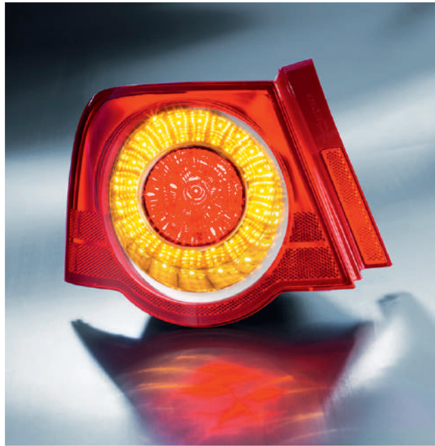
Figure 3.96 Light cluster that uses LEDs
